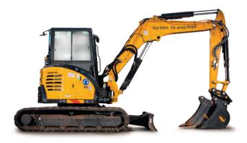
**3T.5T-6T EXCAVATOR**Minor Earthworks, Detailed Excavation,
